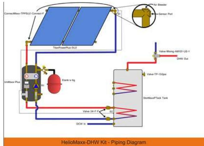
Solar Hot Water Systems, also known as Solar Thermal Systems (STS) operate differently from photovoltaic (PV) systems. Solar thermal systems run water or fluid through their system. The solar panels are heated and the water running through them gets heated, so the water is ready for use.
